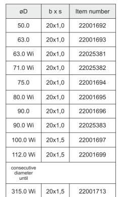
\*) Wi = for folded spiral-seam pipes
